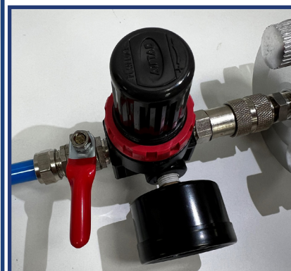
Pressure Regulator, adjustable without a screwdriver
