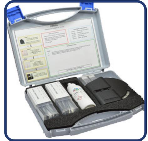
The WTS non-oxidising biocide test kits are based on novel colorimetric or titrimetric procedures and are designed for use by nontechnical persons as a site-based aid. Accurate biocide levels can be measured in minutes to ensure continued system control.
