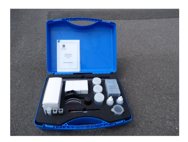
WTS-K101538 Sewage Effluent Residual Chlorine Test Kit
