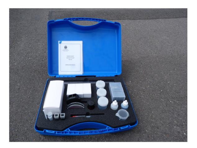
WTS-K101538 Sewage Effluent Residual Chlorine Test Kit 1 x Marine Heavy Duty Case & Foam Insert 1 x Chlorine (Free) LR Comparator Test (0 – 1 mg/l) (100 Tests)
