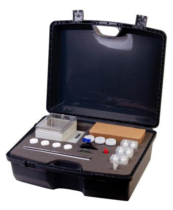
WTS-K100778 Sewage Effluent Test Kit 1 (Complies with MEPC.2(VI)) (Sewage Treatment Plants Installed Prior to 1st January 2010) 1 x Marine Heavy Duty Case & Foam Set 12 x Coliform Bacteria Test (0 – 2424 CFU/100ml) 1 x Total Suspended Solids Test (5 – 500 mg/l) (Unlimited Tests) 1 x Biological Oxygen Demand Test (7.5 – 255 mg/l) (Unlimited Tests) 1 x Spirit Thermometer
